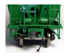
This is one example on how to run the pipe leading to the air hose on freight cars. On locomotives and extra long cars the pipe will need to be run differently. It must end up in the center of the coupler shank. If this is your first time installing these air hoses I recommend installing them on some cars first. They are a little easier to do.
